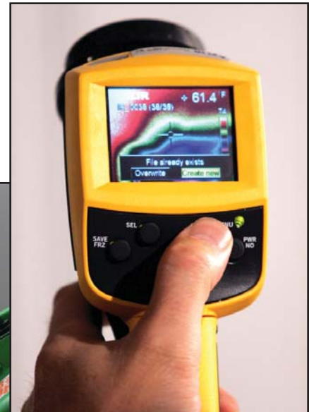
SERVPRO® Professional using a Moisture Sensor and Thermal Camera to detect moisture.
